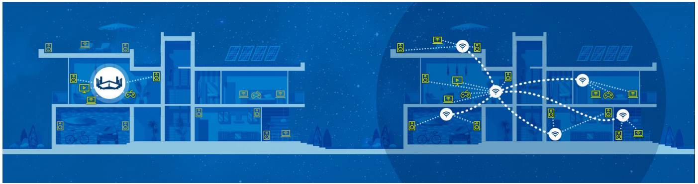
Figure 1. The home network topology is evolving to a home network with multiple access points and extenders with wired or Wi-Fi backhaul.
